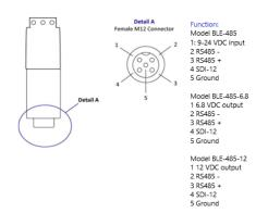
The Anuracom comes with a 5 pole single keyway M12 type A single keyway IP67 female connector designed to mate with a 5 pole field connector with pinout as follows.
