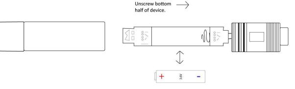
Replace battery from within circuit board.
